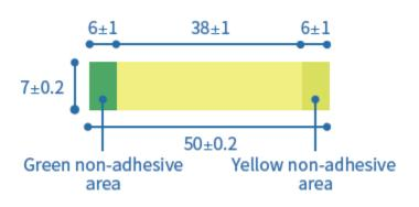
The Label is made of 3 Parts (Yellow Adhesive Tape + Yellow Non Adhesive Tape + Green Non Adhesive Tape) it is used for Fixing and sealing the end of SMT Carrier Tape Reels and other materials Reels.
