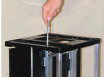
Tighten screws to fix adjustable guide rail unit
