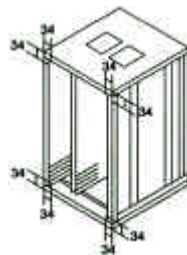
Same reference position for all of the outside corners
