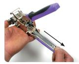
Pull the slider towards the direction of the arrow.
