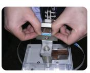
Position two ends of the tapes to be joined onto splice tool.
