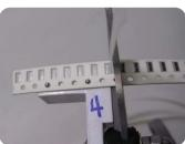
Cut reel using pitch scissor.
