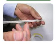
Peel off the reel cover tape to the first component.
